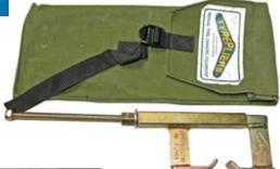
Tyrepliers cannot accommodate 8.00" cruiser rims commonly used with 240mm wide rear tires. Its only other design limitation is that it cannot be used with solid wheels. But for most wheels, the Tyrepliers are the right tool for the job.
